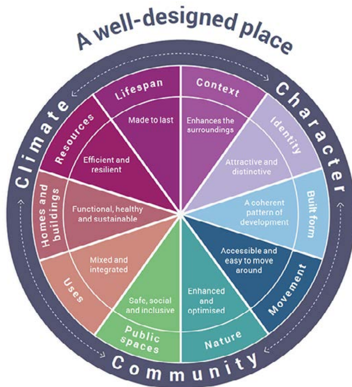
Figure 06: The 10 characteristics of a well-designed place from the National Model Design Code (2021).
